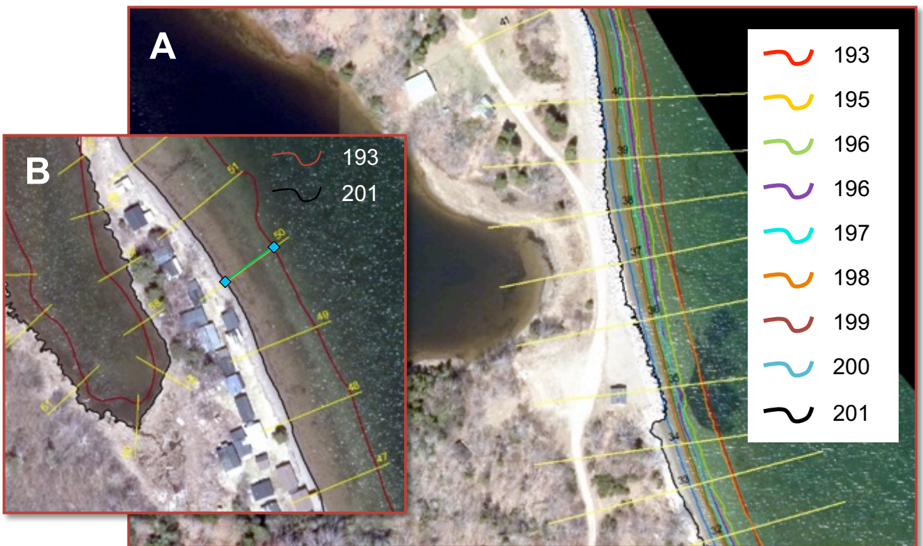
FIGURE 18. Example of the mapped shorelines and transect placement (25 m interval) in part of the Malikewe'j study site (A). Sub-set "B" part of the Potlotek study site shows how the shoreline displacement measurements were taken: the length of the green line represents the total retreat distance of the shoreline from 1939 to 2014.
