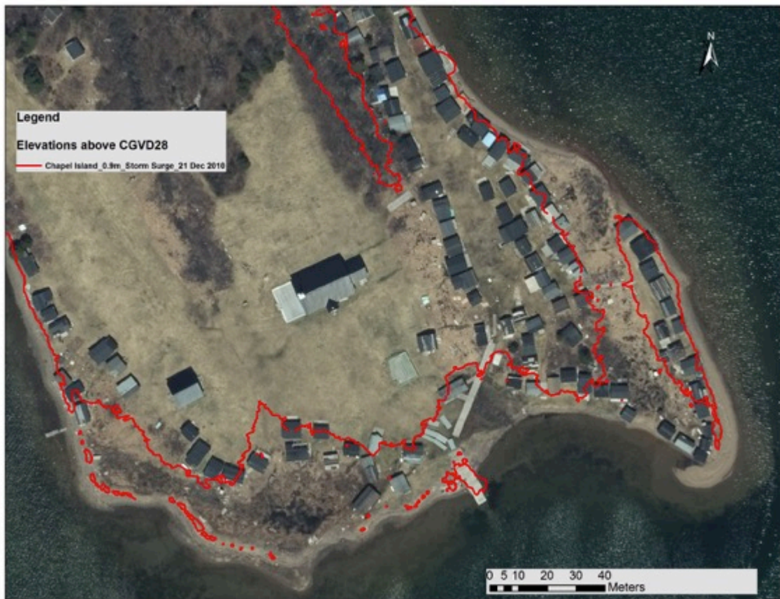
Figure 3 LiDAR aerial photo with 0.9 m CGVD28 red contour depicting 21 Dec 2010 flooding limits
